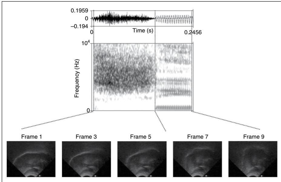
**Fig. 1.** A sample waveform and spectrogram of [ʃi] (top) and ultrasound frames obtained during the acoustic noise period (frames 1–5) and vocalic period (frames 6–9, bottom). Only odd-numbered frames are presented in this figure due to space limitation. In ultrasound images, the tongue back appears on the left, and the tongue tip/blade on the right. A method for visualizing and quantifying tongue shape is explained in the text.
