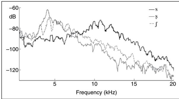
**Fig. 8.** Representative multi-taper spectra of three fricatives /s, ʃ, f/ in the /a/ vowel context taken at mid phase of frication noise.
