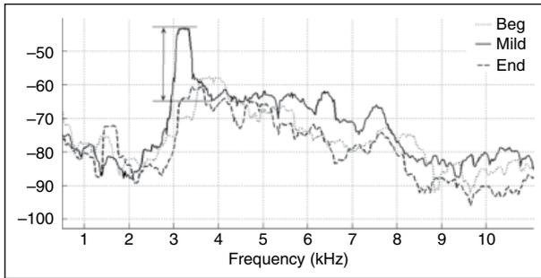
**Fig. 6.** An illustration of a whistled peak produced by speaker S.M. An unambiguous whistled peak is observed for the mid phase of this token: the narrow part of the high-amplitude peak has an amplitude extent greater than 15 dB (indicated with an arrow).
